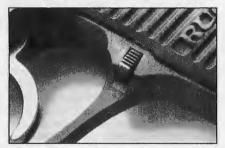
BELOW: SOF Technical Editor Peter G. Kokalis feels the P-85's slide release lever is too long. Slide fails to hold-open after the last round is fired because of thumb pressure on slide stop when Weaver hold is employed. Production series slide stops will be shorter.
